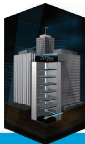
Diagram of fibre connectivity from a Lightspeed distribution point to an office or floor.
